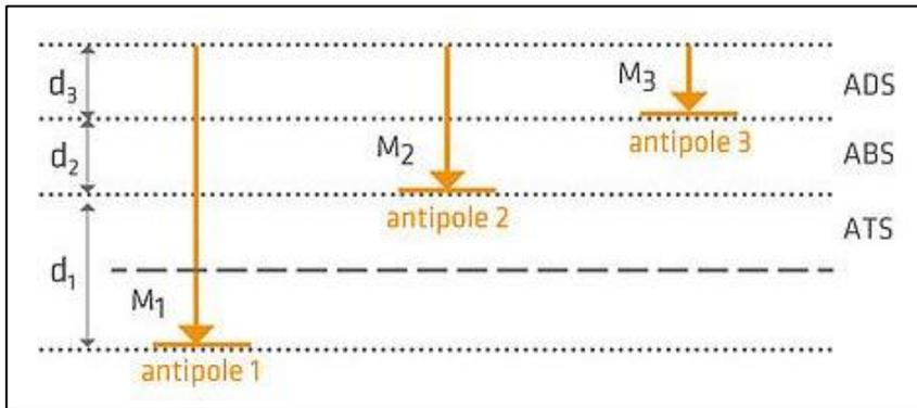
Fig. 7 Calculation of thickness in asphalt pavements
