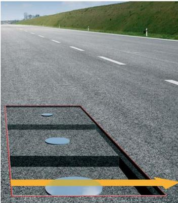
Fig. 6 Measurement path over circular plates
