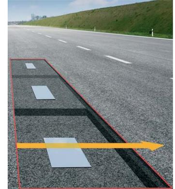
Fig. 12 Measuring path over rectangular reflectors
