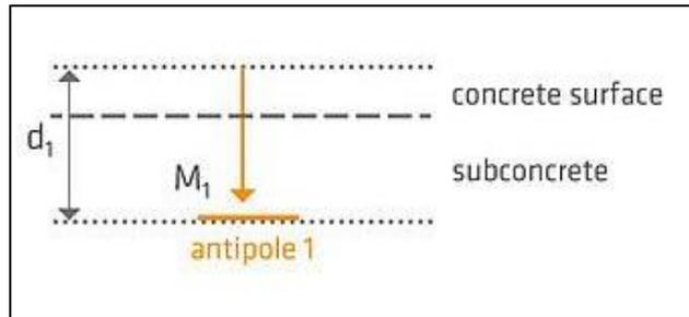
Fig. 11 Calculation of thickness in concrete pavement
