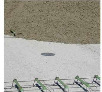
Fig. 10 Steel reflector plate
