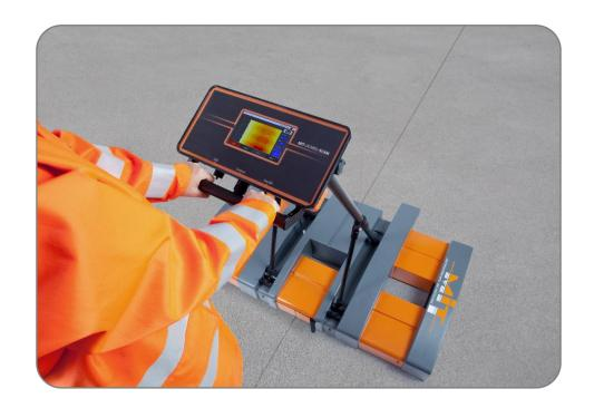
The dowel position measuring system **MIT-**DOWEL-**SCAN** is designed in compliance with ASTM E 3013 and affords the nondestructive and accurate testing of dowel and tie bar positions in concrete roads and areas.
