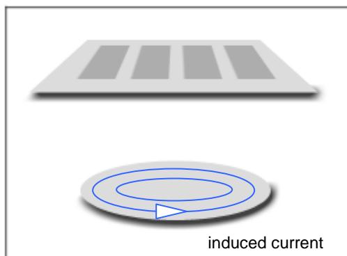
At the bottom of the layer is a reflector (a foil or circular plate of metal). The pulsating magnetic field induces eddy currents in the reflector which subside exponentially and in turn generate a time-dependent magnetic field: the so-called response field.
