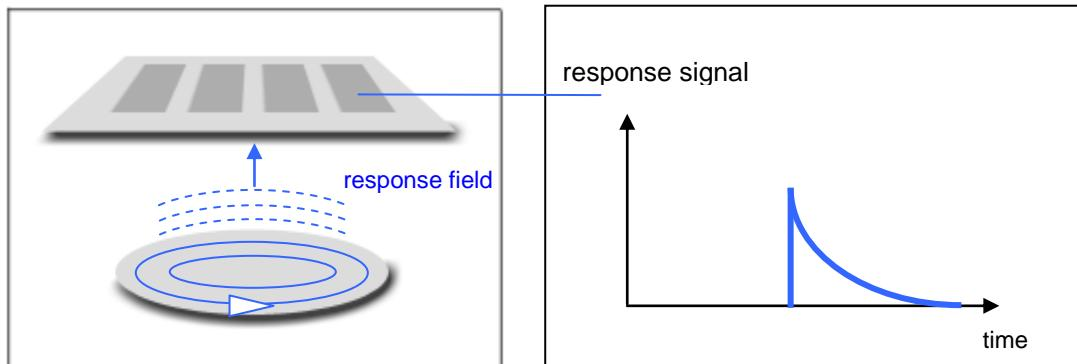
The emission field is generated by alternately switching the current on and off in very short intervals (in the range of a few microseconds). Once the emission field has completely subsided the response field is measured. In this way an overlap of the response signal and the comparatively strong emission
