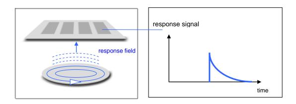
The emission field is generated by alternatingly switching the current on and off in very short intervals (in the range of a few microseconds). Once the emission field has completely subsided the response field is measured. In this way an overlap of the response signal and the comparatively strong emission
