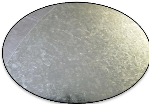
Figure: Example of a circular Sendzimir-galvanized circular steel plate
